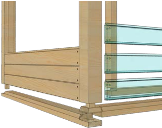
POST AND BEAM SYSTEM
